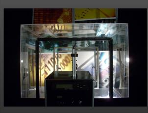
App-Lab's Lift Performance Tester is a test and measurement instrument to characterize the performance and efficiency for combinations of propellers and motors used on drone sized aerial vehicles such as multi-copters and airplanes.
